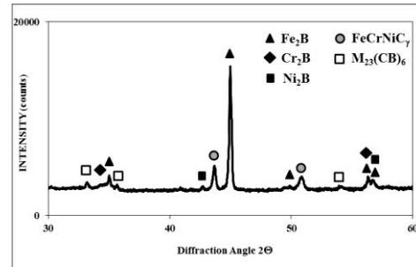
Fig. 5. XRD patterns of laser-borided 316L steel
