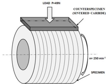
Fig. 3. Scheme of wear test.  $P = 49 \text{ N}$ , rotational speed  $n=250 \text{ min}^{-1}$
