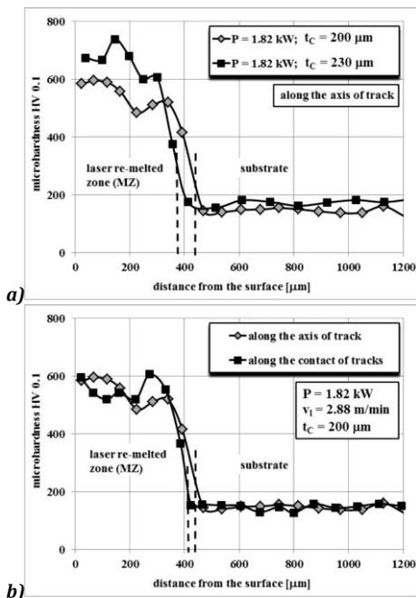
Fig. 7. Microhardness profiles of laser-borided layer formed on 316L steel: along the axis of track at various thickness of paste coating  $t_c$  (a), at the thickness of paste coating  $t_c = 200 \mu\text{m}$ , depending on the measurement place (b)
