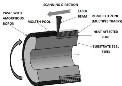
**Fig. 1. The two-step method of laser-boriding**
