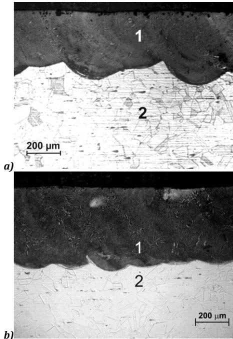
Fig. 4. Microstructure of laser-borided 316L steel at laser beam power of 1.82 kW using paste coating with thickness: 230  $\mu\text{m}$  (a) and 200  $\mu\text{m}$  (b); 1 - remelted zone (MZ); 2 - substrate
