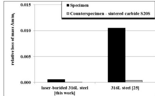
Fig. 8. The results of wear resistance tests
