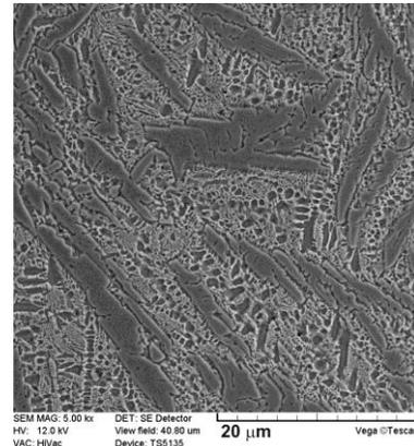
Fig. 6. SE image of re-melted zone (MZ). Hard ceramic phases (iron and chromium borides) in a soft austenitic matrix
