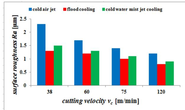
Fig. 10. Influence of cooling technique on surface roughness *Ra*. Elaborated on the basis of [1]
