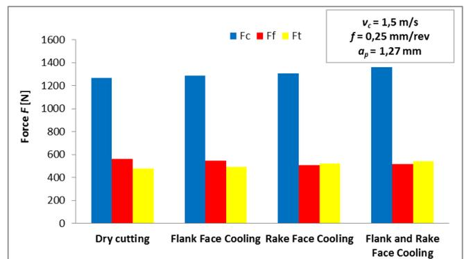
Fig. 4. The influence of cooling technique on cutting forces values. Elaborated on the basis of [9]
