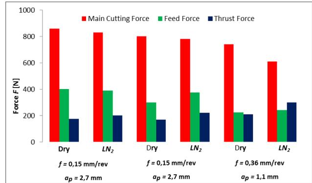
Fig. 2. Cutting forces values for variable feed rate and depth of cut values after dry and cryogenic machining. Elaborated on the basis of [2]
