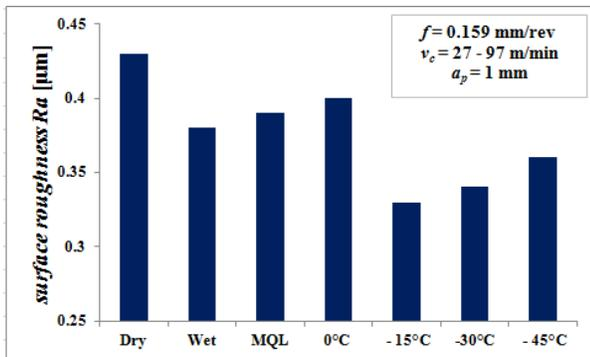
Fig. 9. Influence of the machining technique on surface roughness. Elaborated on the basis of [31]
