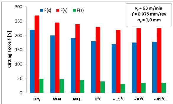
Fig. 5. The influence of cooling technique on cutting forces values during milling of titanium alloy. Elaborated on the basis of [31]
