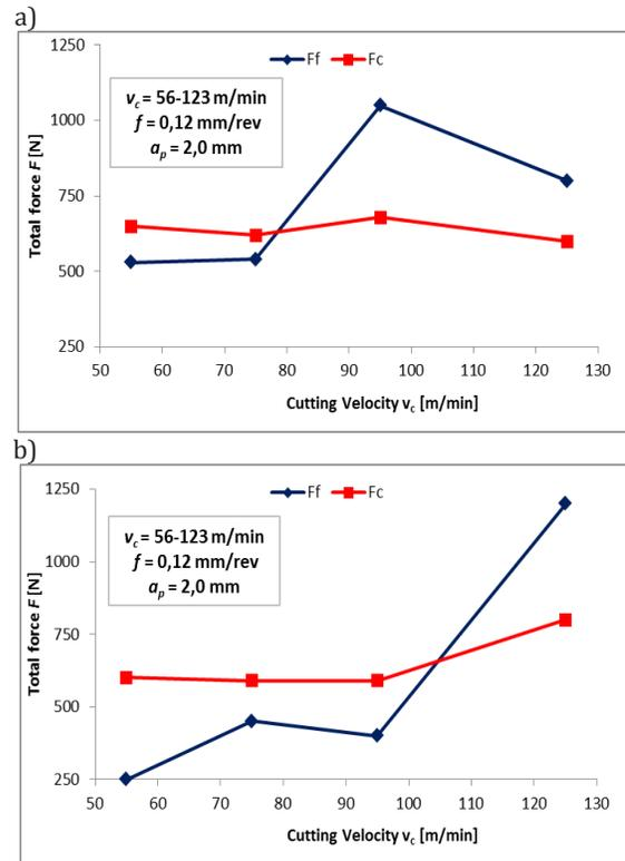
Fig. 7. Cutting forces values in function of cutting velocity during: a) dry and b) cryogenic machining. Elaborated on the basis of [24]
