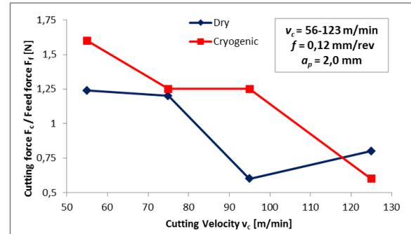
Fig. 6. Force ratio values in function of cutting velocity during dry and cryogenic machining. Elaborated on the basis of [24]
