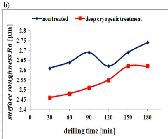
**Fig. 11. Surface roughness parameter  $R_a$  values measured: a) on base of blind hole with drilling time, b) on side wall of blind hole with drilling time. Elaborated on the basis of [21]**
