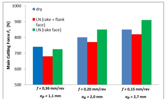
Fig. 3. Main cutting force for different cooling conditions. Elaborated on the basis of [2]
