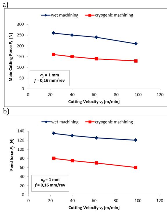
Fig. 1. Main cutting force (a) and feed force (b) values in a function of cutting velocity. Elaborated on the basis of [6]
