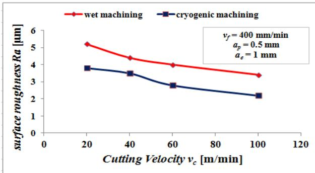
Fig. 8. The influence of machining method on surface roughness parameter *Ra* value for *Ti-6Al-4V* alloy. Elaborated on the basis of [6]
