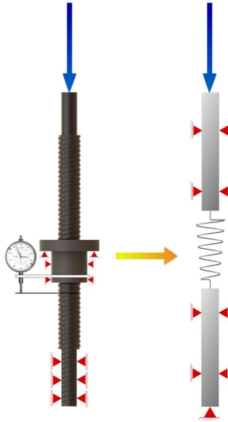
Fig. 5. Diagram of ball-screw mechanism modeling adopted in the identification process
