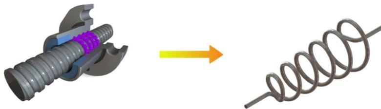
Fig. 2. Modeling ball-screw mechanism by replacing the mechanism with a spring element
