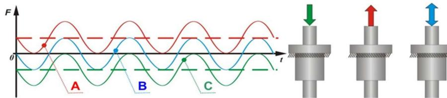
Fig. 4. A diagram of three variants of load on the ball-screw mechanism during the experiment
