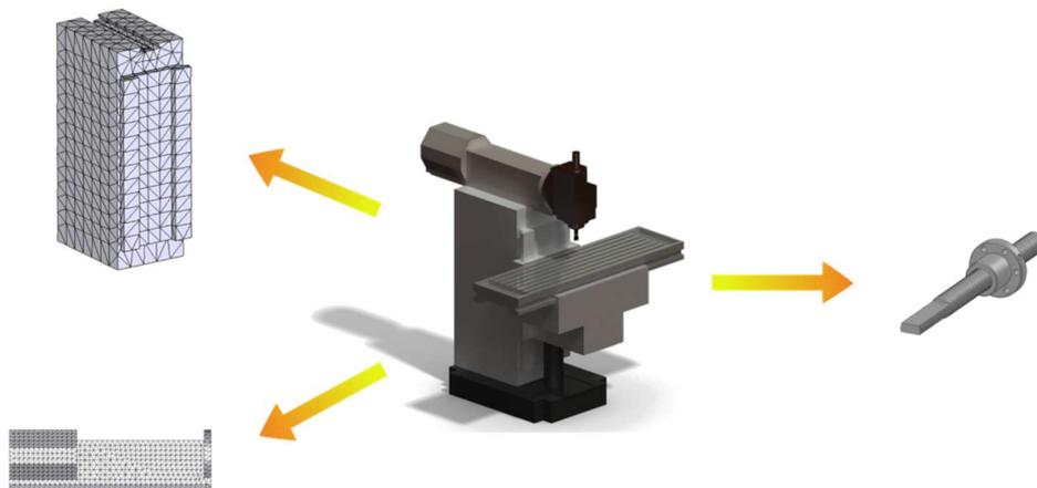
Fig. 1. The concept of modeling load-carrying systems in machines containing ball-screw mechanisms
