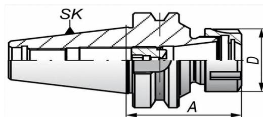
c) Clamping holders (for ER DIN 6499 sleeves) for tools with cylinder grips BT-ER | TYPE 7626 [7]
