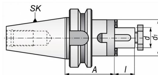
b) Universal milling arbors for milling cutters with locking grooves or drive grooves DIN 138BT-DC | TYPE 7361 [6]
