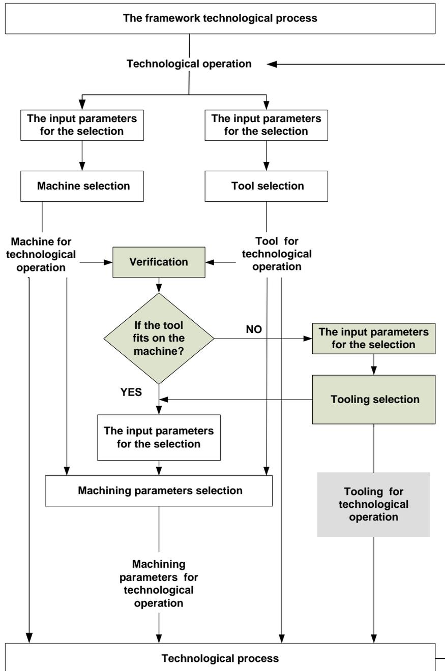
Fig. 2. Position of the tooling selection in the design of the technological process
